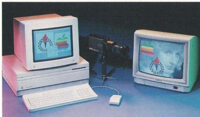
RSVP Publisher uses a video camera or VCR to capture images that you can then manipulate before incorporating them into text documents.
